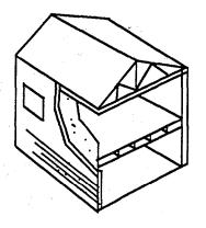
WOOD ROOF, WALLS AND FLOORS PROTECTED BY 1/2" GYPSUM BOARD
